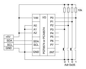
More significant bits of this microcircuit can be used, for example, for LED control. Then it is always necessary to set less significant bits in a high level.
